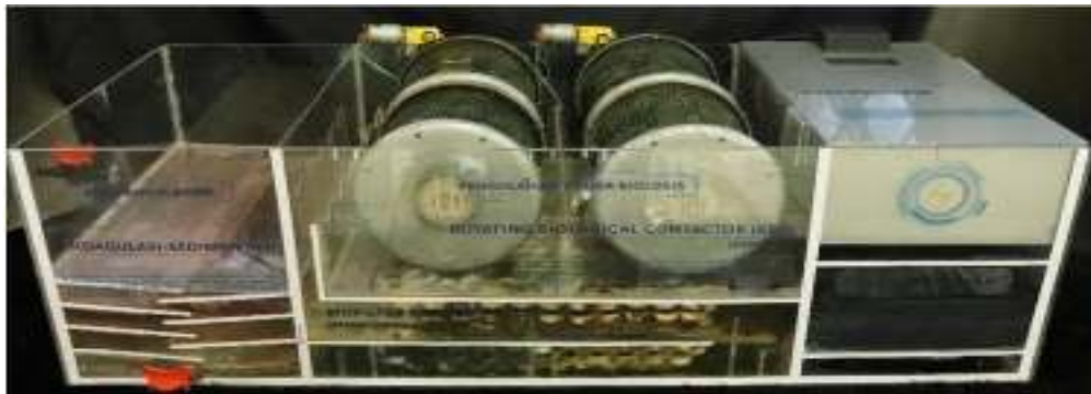
Gambar 1. Reaktor Pengolahan Limbah Cair Tekstil Berbasis Hybrid Attached Growth Biofilm Terintegrasi Arduino (Rahmadi et al. (2022)).
