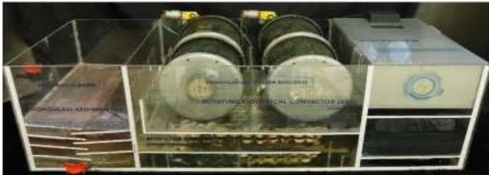
Gambar 1. Reaktor Pengolahan Limbah Cair Tekstil Berbasis Hybrid Attached Growth Biofilm Terintegrasi Arduino (Rahmadi et al. (2022)).
